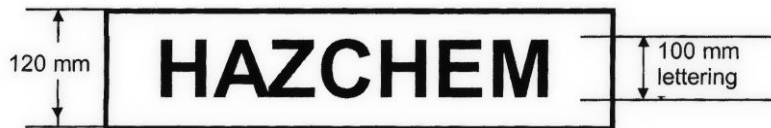
Fig TO5.3 Hazchem Placard (Outer Warning Notice)
